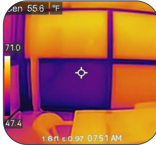
Existing: 1" IGU Graylite II SB60
