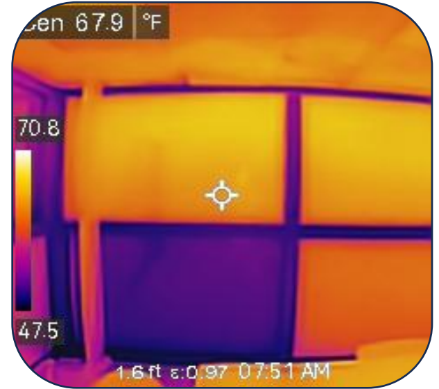
New: 10mm Entermal VIG 366 Clear EFCO Secondary Window System
